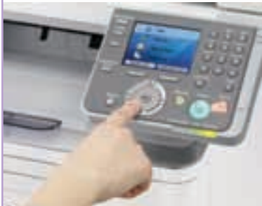
Control Panel with Scroll Wheel
